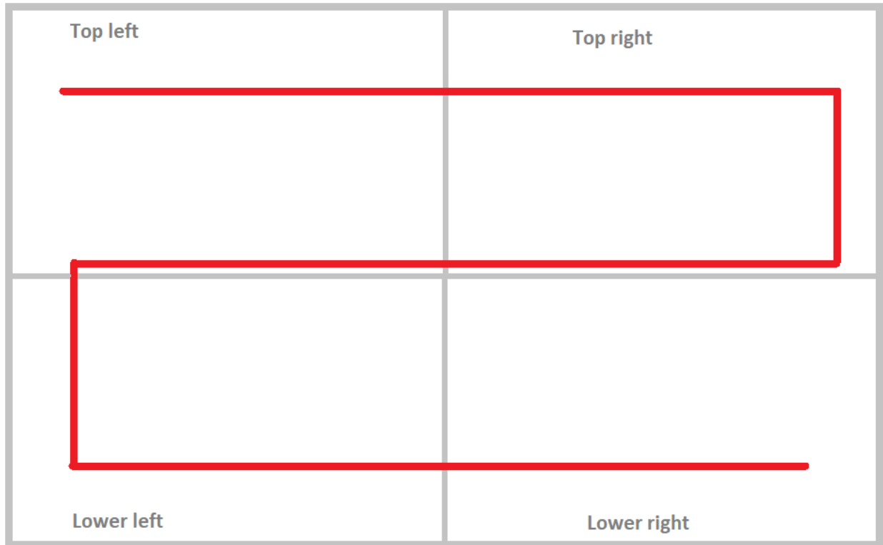
The red rope line on the fish pen netting. The gray lines will be the PVC framework.
