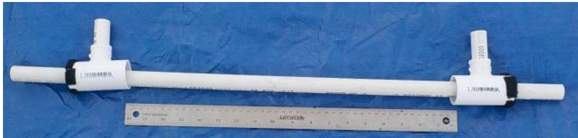
Both wet-mateable connectors on the new section of cable. Note that the Velcro loops on both the cable and connectors will provide enough friction to hold the wet-mateable connectors onto the cable during transport, but still allow ROVs to slide the connectors along the pipe.
