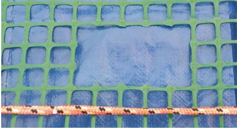
A damaged area of the fish net pen.
