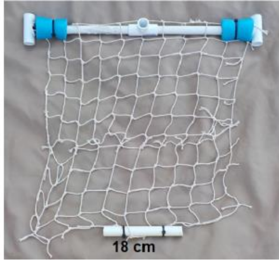
Left: The decorative cloth netting of the ghost net. Right: The decorative cloth netting is attached to the framework. Flotation is added to the top, and an 18 cm length of PVC is added to the bottom of the net for weight.
