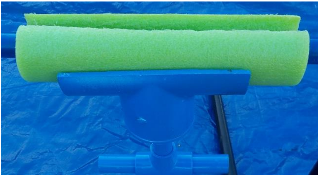
The failed buoyancy module attached to the array cable. Note that the buoyancy module is positively buoyant in water and will stay positioned on the underside of the array cable.
