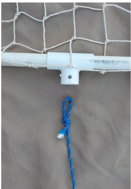
Left: The ghost net is attached to the rope. Right: The pin runs through the \frac{1}{4} " holes in the PVC tee and through loop in the rope. The other end of the rope attaches to the inter-array cable.
