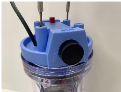
Pressure relief system made with rubber stopper. 1
