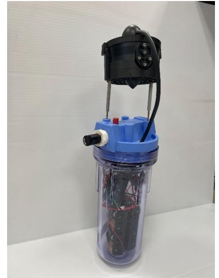
The Molokini showing the thruster mount, switch, wiring, and housing. 1
