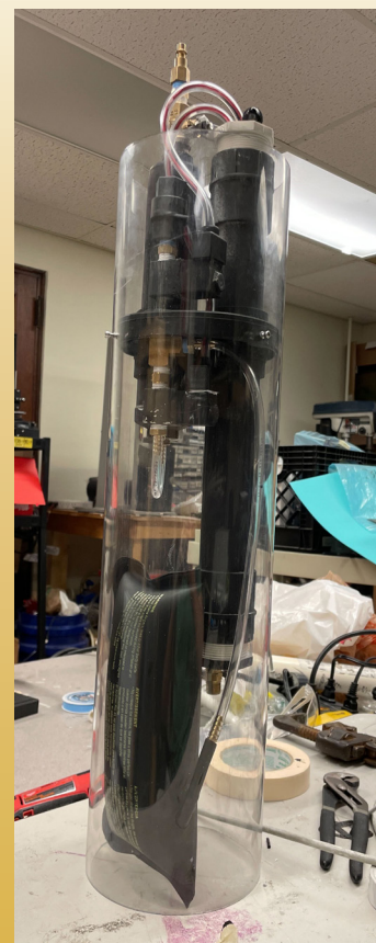
Fig. 1 - Assembled Vertical Profiling Float
