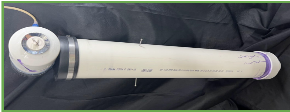
Figure 1. SEAL Robotics Vertical Profiling Float with battery compartment on top.
