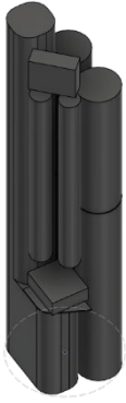
Figure 2 – Float concept CAD (internals only, some parts modelled to low degree of accuracy)
