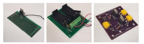
microcontroller. We used two transistors as switches for the two pumps but considered relays as well. We went through several PCB variations and microcontrollers before settling on our current design.
