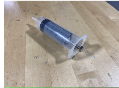
Buoyancy motor of the float Photo Credit: Dwayne Wallace
