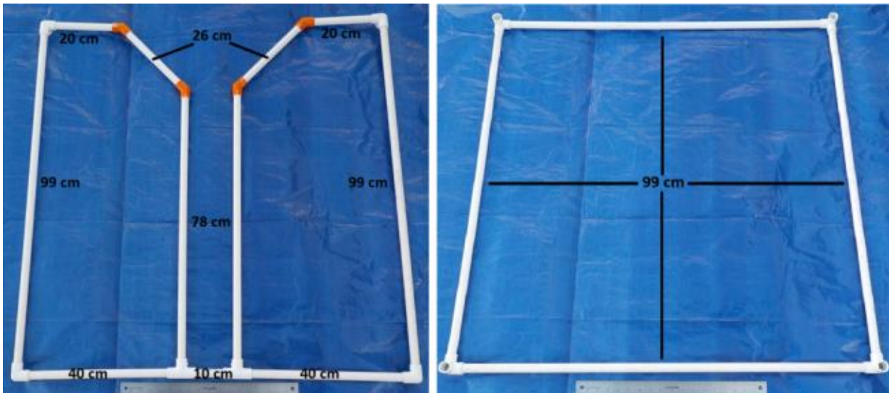
Left: The top of the docking bay constructed from ½-inch PVC pipe. Right: The base of the docking bay constructed from ½-inch PVC pipe.
