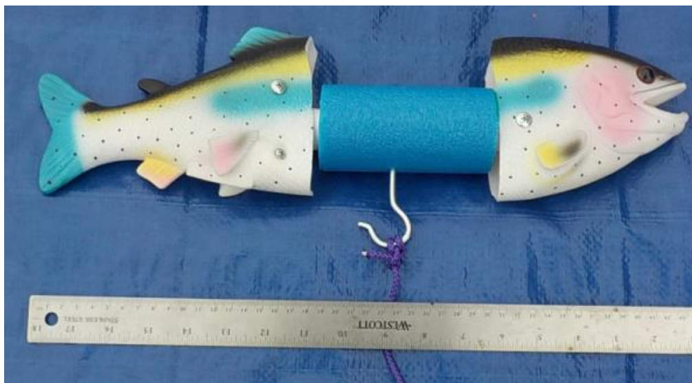
Foam flotation is added to the ½-inch PVC pipe. A #6 screw hook passes through the foam flotation and is attached to the variable length of PVC pipe. A rope is attached to the screw hook. The other end of the rope is attached to a weight.
