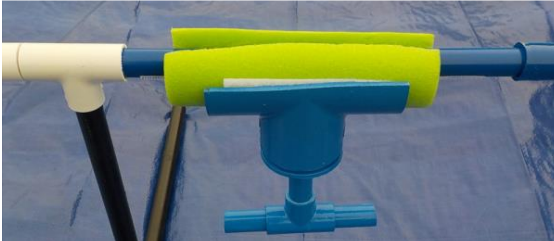
The new buoyancy module secured to the inter-array power cable. The Velcro loops inside the foam flotation are attached to the Velcro hooks on the bottom of the cable.
