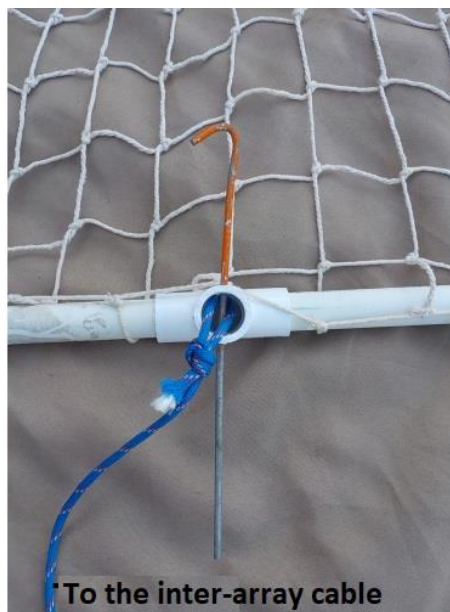
Left: The ghost net is attached to the rope. Right: The pin runs through the \frac{1}{4} " holes in the PVC tee and through loop in the rope. The other end of the rope attaches to the inter-array cable.
