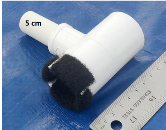
A wet-mateable connector constructed from a 1-inch x 1-inch x 1/2-inch tee .
