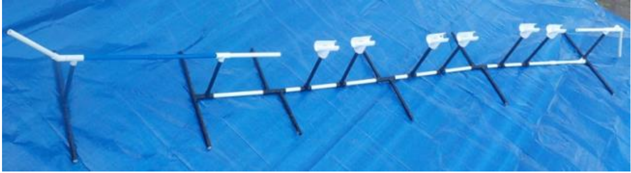
All five stands connected together. Note that 3/8-inch rebar inserted inside the central PVC pipes of the inter-array cable stands will provide weight and stability to the stands.
