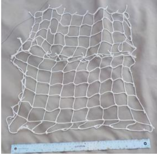
Left: The decorative cloth netting of the ghost net. Right: The decorative cloth netting is attached to the framework. Flotation is added to the top, and an 18 cm length of PVC is added to the bottom of the net for weight.
