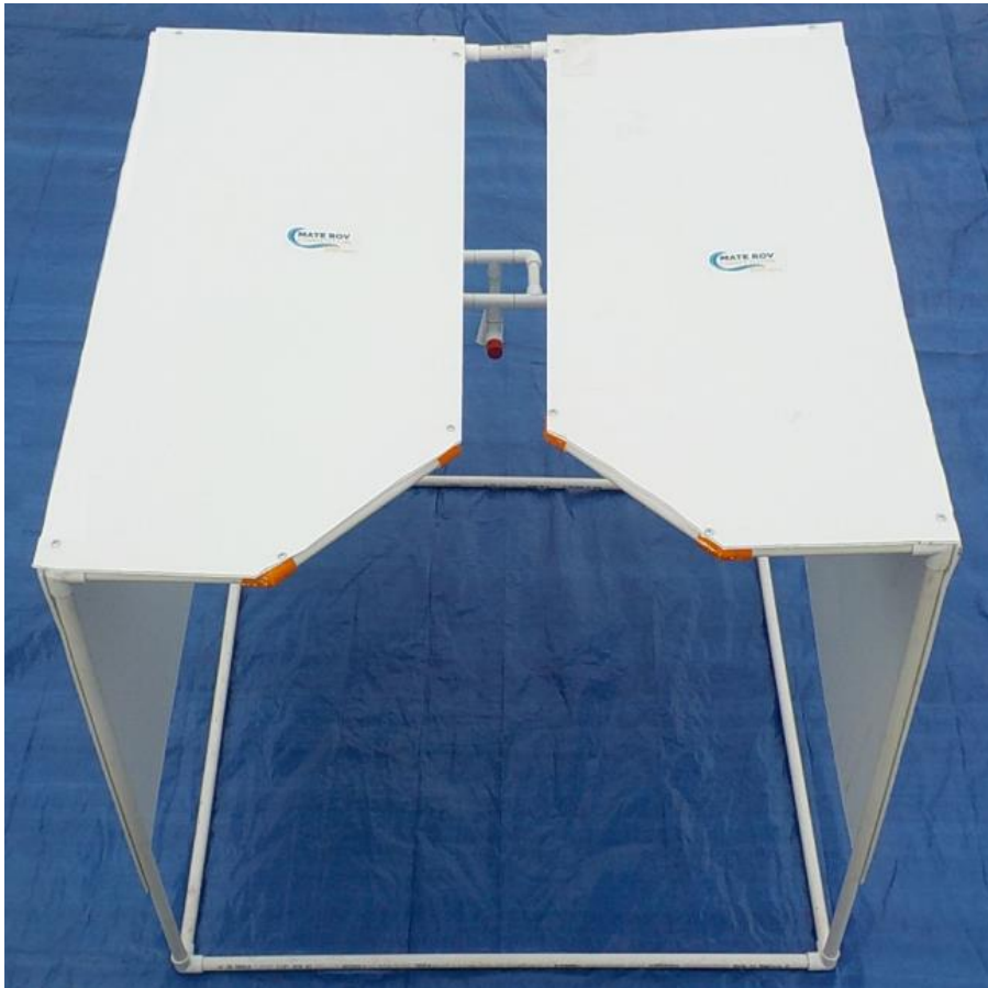
The docking bay with corrugated plastic sheeting attached.
