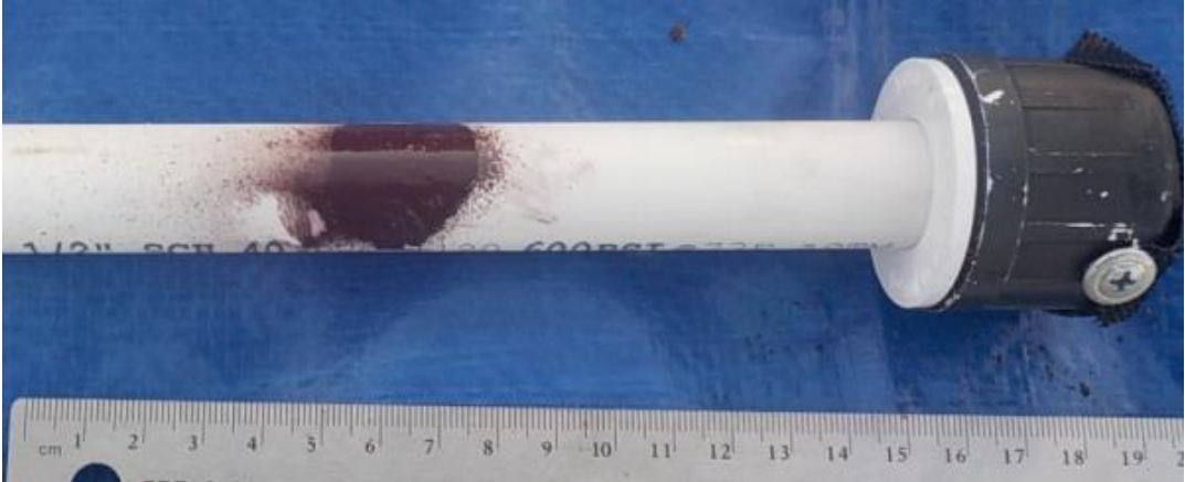
The damaged section of the inter-array cable. The damaged section is a spot of brown paint at least 1.5 cm in diameter.
