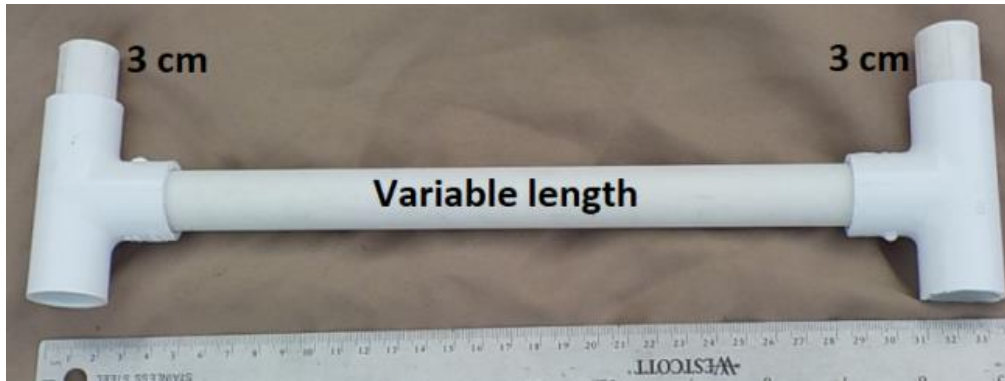
The variable length of ½-inch PVC pipe for the fish.
