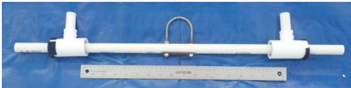
Both wet-mateable connectors on the new section of cable. Note that the Velcro loops on both the cable and connectors will provide enough friction to hold the wet-mateable connectors onto the cable during transport, but still allow ROVs to slide the connectors along the pipe.
