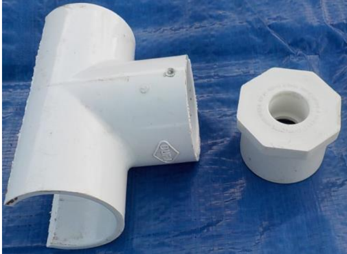
A 1 ½-inch to ½-inch reducer bushing is used to connect the cradles to the stand.
