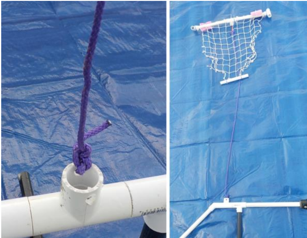
The ghost net secured to the inter-array cable
