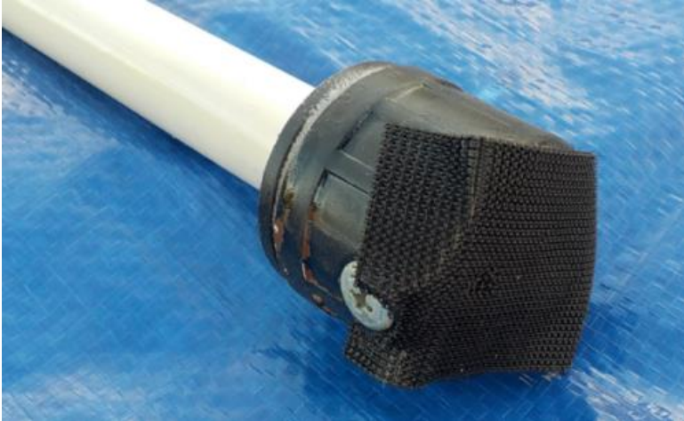
1-inch end cap covered with Velcro hooks. A 1-inch to ½-inch reducer bushing is used to connect the end cap to the ½-inch pipe. Note that screws are used to secure the Velcro to the end cap.
