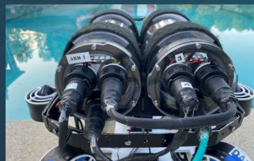
Figure 2: ROV frame showing Bulgin connectors.
