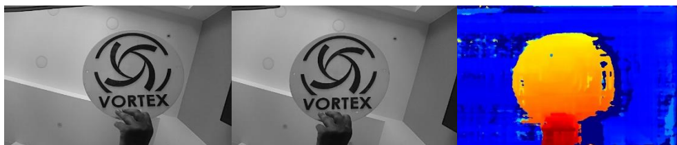
Figure 38: left, right and disparity frames.
