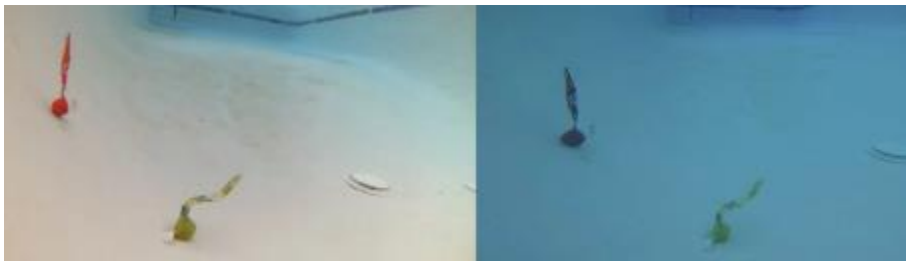
Figure 13: The Picture on the left was taken with the Explore HD 2.0 camera, the one on the right, with our old fish-finder cameras.
