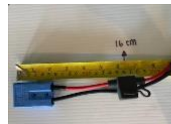
Figure 11: 25 Amp Fuse 16 cm from main power.
