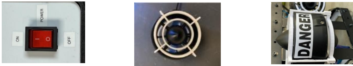
Figure 18: Safety features include safety on/off switch, shroud, guards, and danger stickers on all thrusters.
