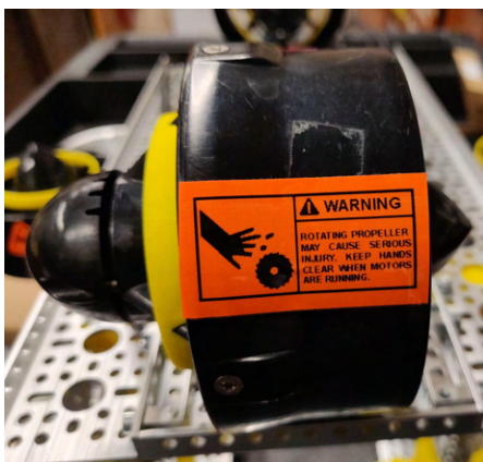
Figure 19B (above): Warning labels on thrusters follow ANSI Z535.3-2011 for safety symbols (ANSI, 2011).
