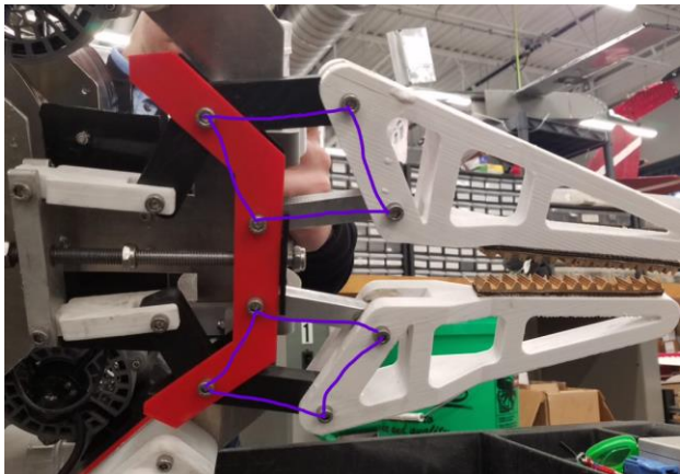
Figure 5: Robot gripper with four-bar linkages outlined
