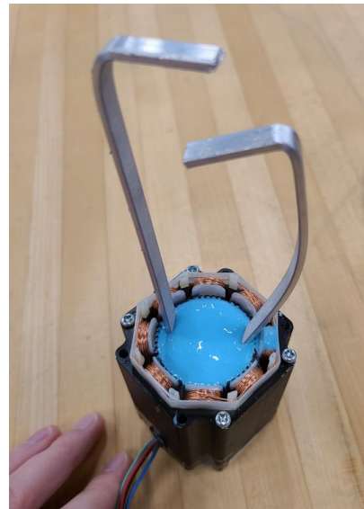
Figure 6: Silicone mold filling the motor voids
