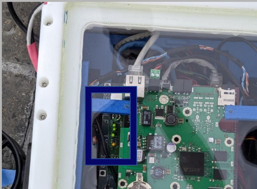
Figure 2: Indicator Light Through Acrylic Window
