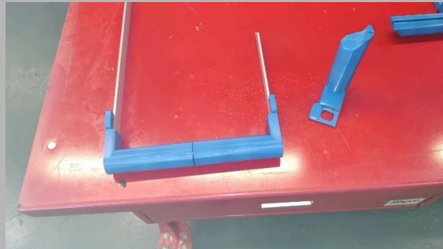
Figure 16: Handles Being Connected Using Aluminum Bar
