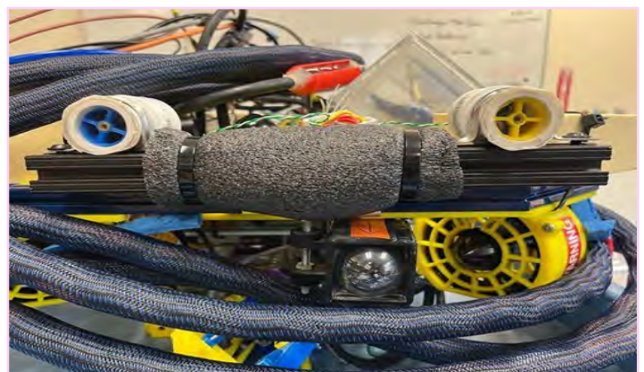
Figure 18: Second prototype of laser rangefinder, mounted on ROV.
