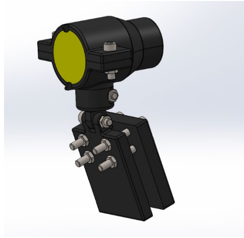
Figure 17: CAD model of 3D printed camera mount prototype
