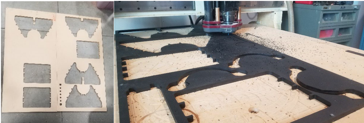
Figure 2: Frame cut from single sheet of pressed wood (left) and HDPE (right) using CNC machine.
