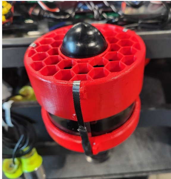
Figure 18: Thruster shrouds designed to prevent injuries caused by thruster blades.
