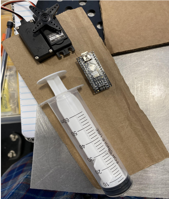
Figure 6: Layout testing for the float, with the syringe, circuit board, and motors present
