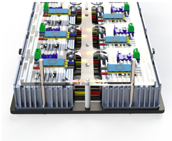
Figure(17) : ESC and Current sensor over each Converter
