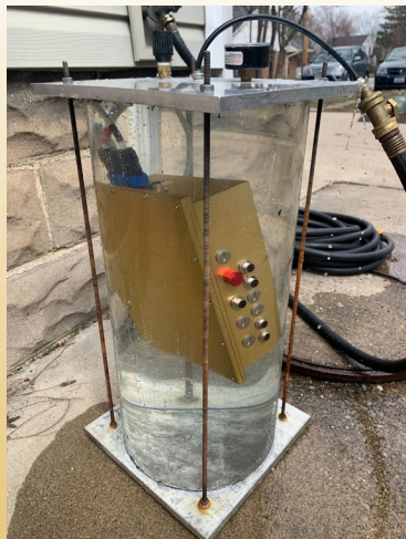
Fig. 2 - The Company's Pressure Testing Chamber During Testing of the Power Box Outside
