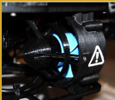
Fig. 4 - A Thruster, Featuring Custom-Printed Ducts with Integrated Safety Shrouds and Warning Placard
