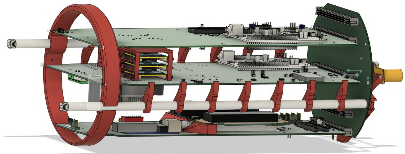
**Figure 21:** Onboard electronics in the electrical housing.
