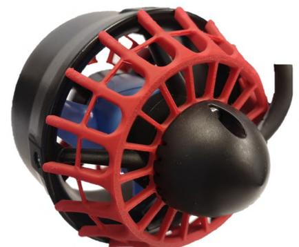
Figure 5: Front side of T200 thruster with thrust guards.
