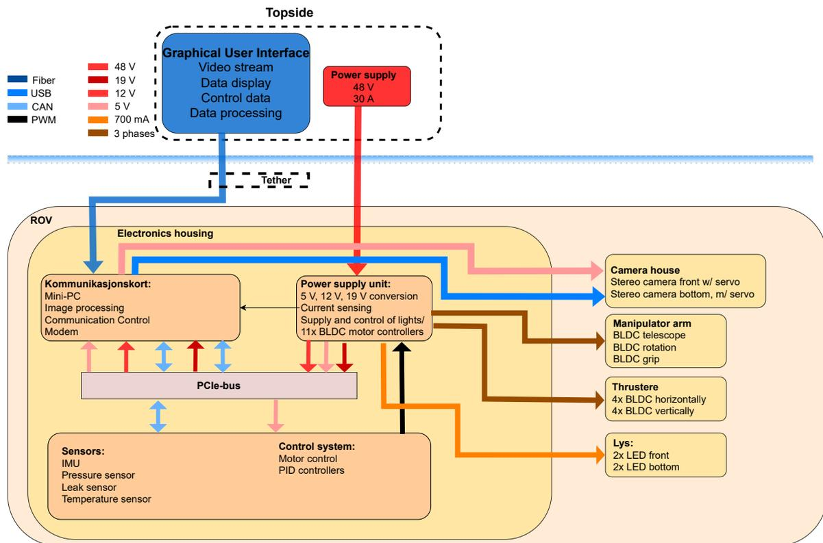
Figure 16: Simplified block diagram of the ROV.
