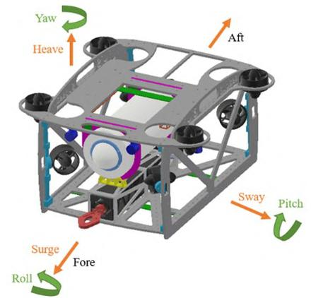
**Figure 9:** The six degrees of freedom for an ROV.
