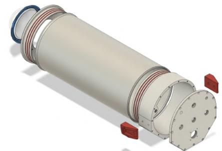
**Figure 7:** Exploded view of the electronics housing.
