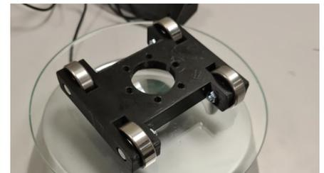
**Figure 10:** Supportwall for the manipulator arm.
