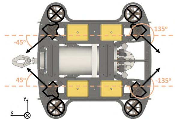
**Figure 6:** Thruster configuration.
