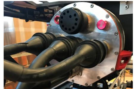
**Figure 18:** Connectors used to supply power to and data from external electronics.
