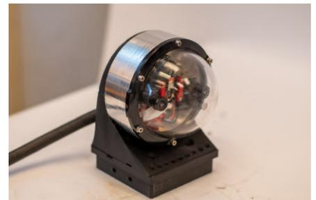
**Figure 19:** External camera house with stereo camera. Camera type: ELP960p. Maximum resolution: 2560x960. Camera sensor: OV9750.
