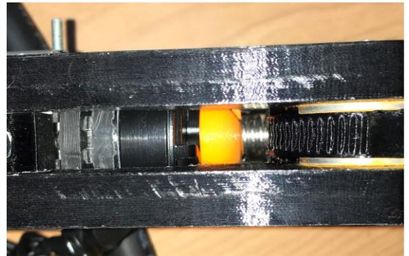
**Figure 13:** Worm gear, motor and worm wheel on the gripper.
