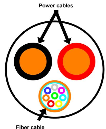
Figure 17: Illustration of the tether used.
