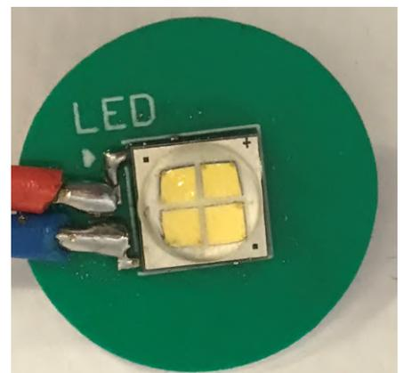
**Figure 20:** LEDs making the external light sources on the ROV.
