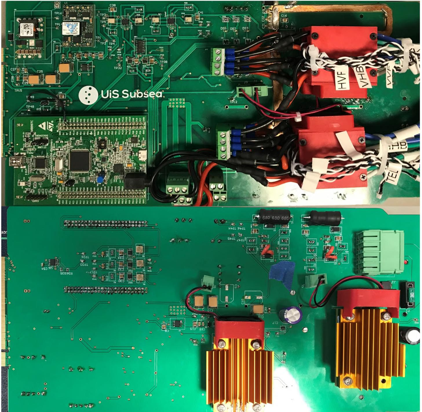
Figure 23: Power supply unit PCB.
