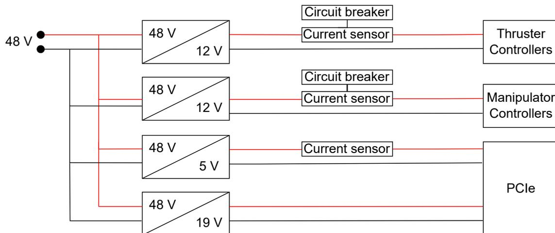
**Figure 22:** Block diagram of the power supply unit.
