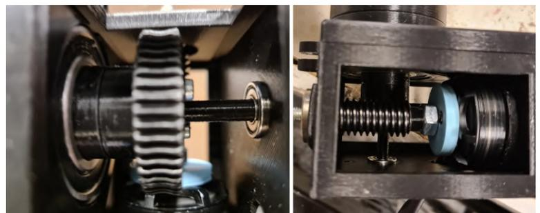
**Figure 11:** Worm wheel (left) and worm gear (right) to rotate the gripper.
