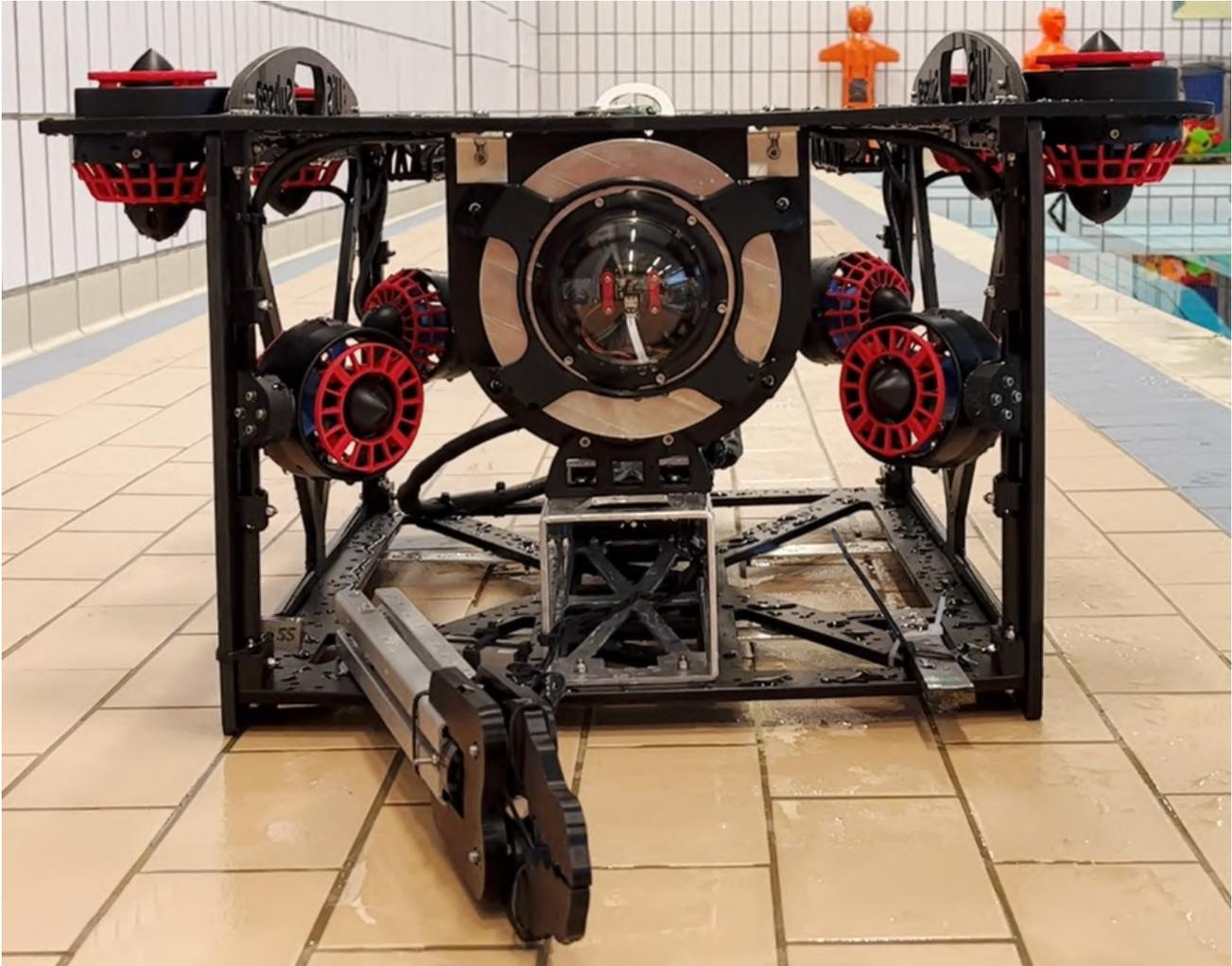
**Figure 2:** Fenris shown from the front with the spare manipulator arm mounted.
