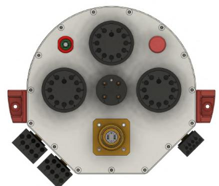
**Figure 8:** All connectors that are used on the ROV. Mounting brackets are also shown.
