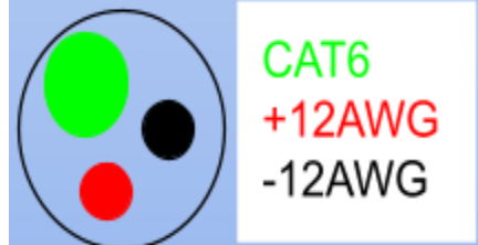
Fig. 23 - Tether cross section.
