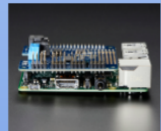
Fig. 24 - Raspberry Pi plus Adafruit shield stack.
