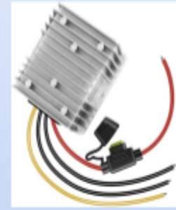
Fig. 21 - Buck converter: 48V to 12V.
