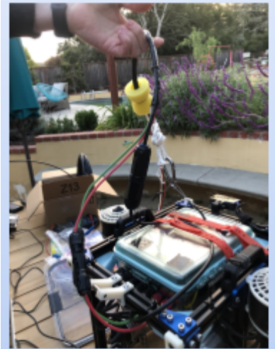
Fig. 2 - Tether strain relief.
