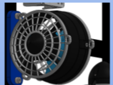
Fig. 4 - 3D printed thruster shrouds.
