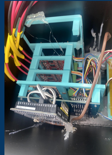
Pictures on the left: four buck converters, one is for the arduino (12V>9V) the other three are for the H-Bridges (12V>7.5 - 12V) Picture on the right: Shows the arduino board, the RS485, the custom controller board, and the three H-Bridges.
