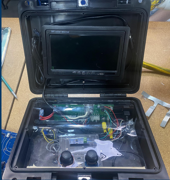
Picture on the left: Control box
