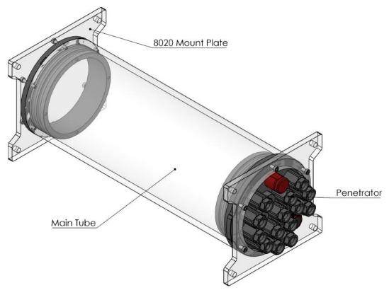
Figure 5: Main electronics enclosure
