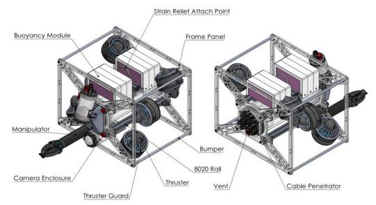
Figure 4: An overview of the mechanical design of the Boxfish
