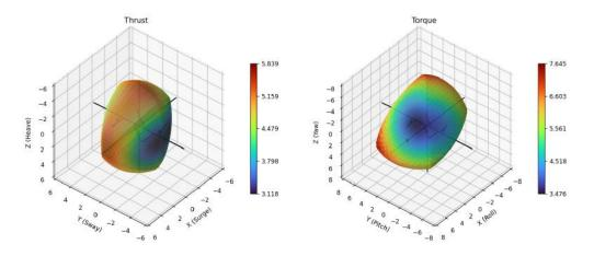
Figure 6: Thrust and torque space of the Boxfish as shown by TAU
