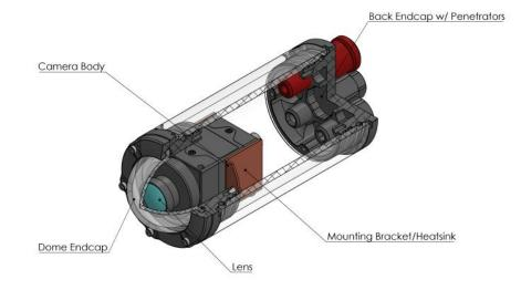
Figure 8: A cutaway diagram of the Boxfish's camera enclosure
