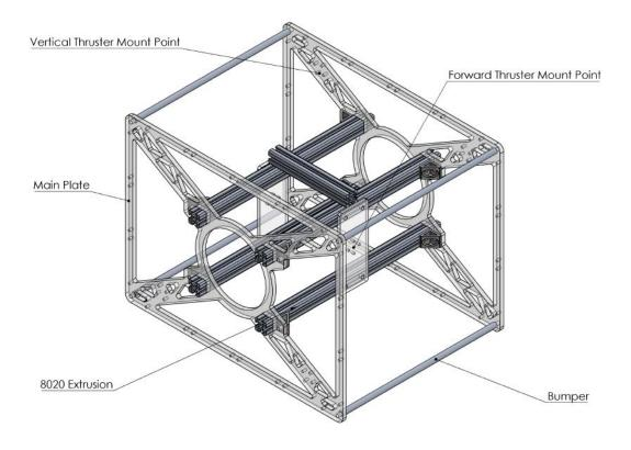
Figure 7: The external frame of the Boxfish
