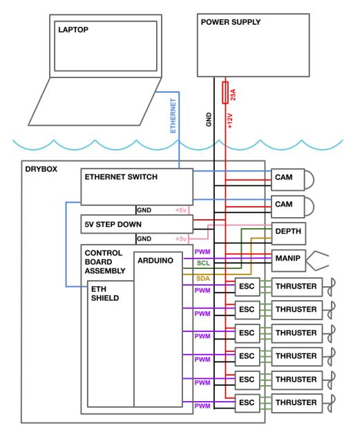
Figure 11: ROV Electronics SID
