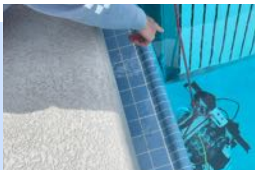
Figure 35: Team member identifies points of leakage in the submerged ROV at a given depth
