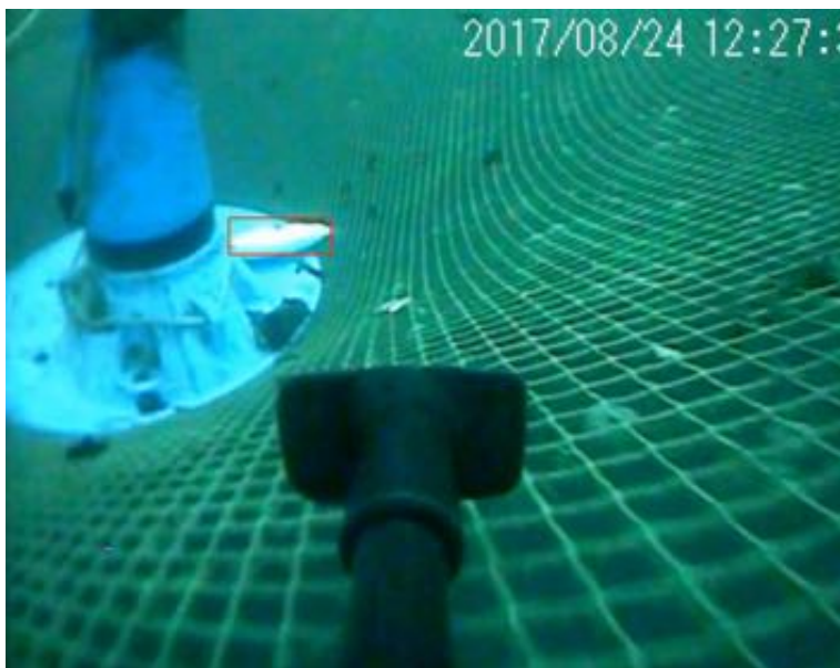
Figure 32: Screenshot of mort detection algorithm output
