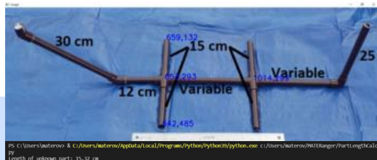
Figure 30: Measurement system being tested on sample shipwreck prop image
