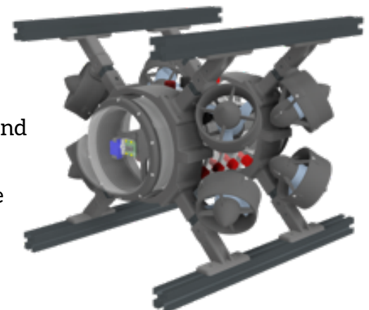
Figure 11: CAD of the ROV's frame
