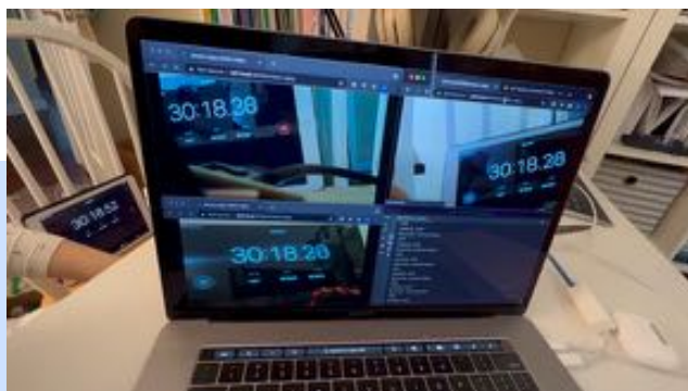
Figure 24: Testing the latency of camera system prototype
