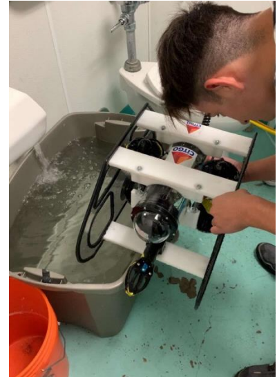
Figure 20: Setup of measuring the buoyancy- photo by Jaziel Gonzalez
