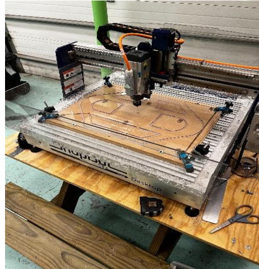
Figure 4: CNC Machine cutting out the ROV's frame
