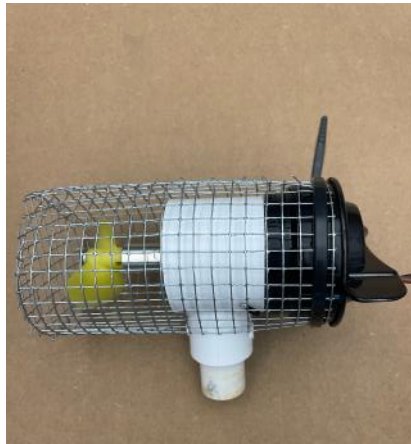
*Image 1: Pasti Dip drying onto Chicken Wire to cover the sharp edges
