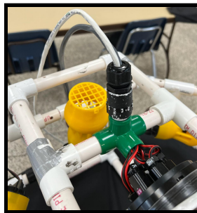
Figure 7. The image above shows the relief system for A.R.R.E.'s tether. This relief prevents the tether disconnecting from the ROV.
