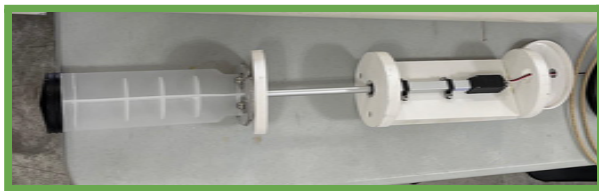
Figure 16. SEAL Robotics Vertical Profiling Float internals - linear servo and syringe plunger.
