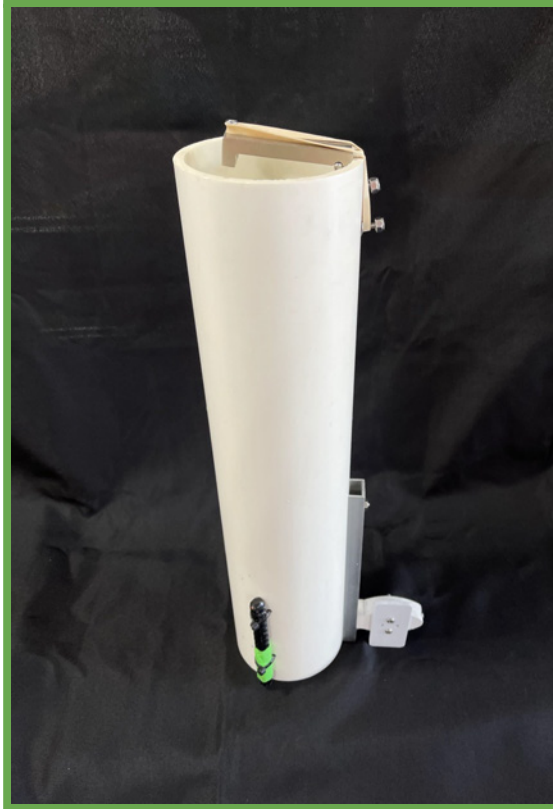
Combo tool for ghost net pin removal and retrieval of the net.
