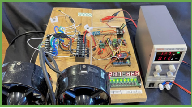
Figure 22. Thruster testing jig used to measure power consumption and to analyze the effects of different precision mode settings.
