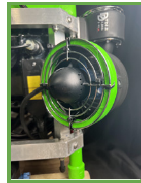
Figure 20. Safety shrouds installed on all thrusters.
