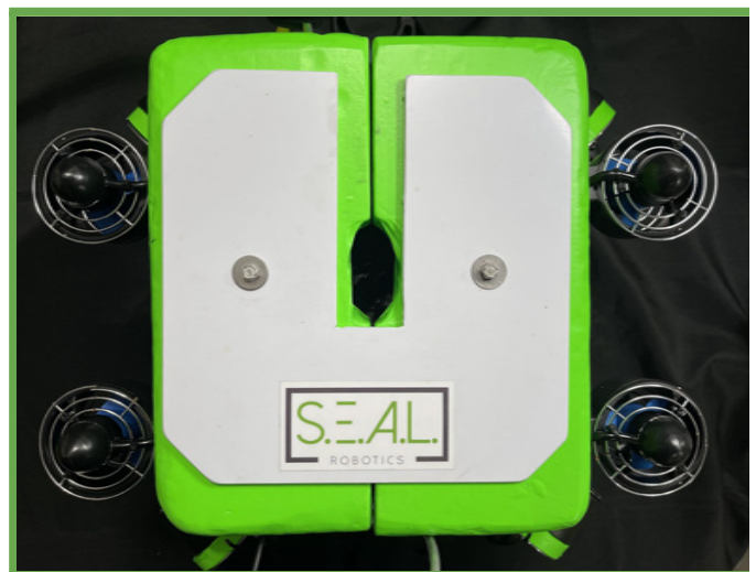
Figure 5: SEALbot overhead view showing the 4 small DiamondDynamics Vertical Thrusters.
