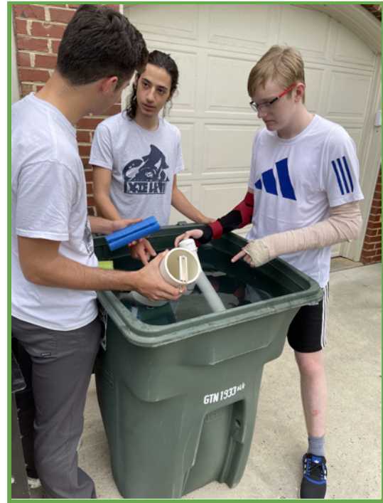
Figure 25. A 90 gallon trash can filled with water may be our most indispensable testing tool, testing everything: thruster power, cameras, sensors, mission tooling, PID software, depth sensors, Profiling Float.
