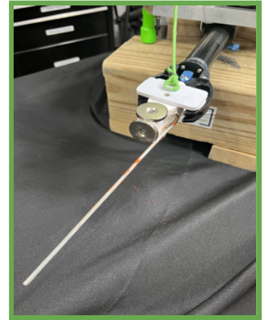
Combo tool for ghost net pin removal and retrieval of the net.
