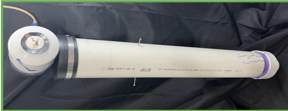
Figure 15. SEAL Robotics Vertical Profiling Float with battery compartment on top.
