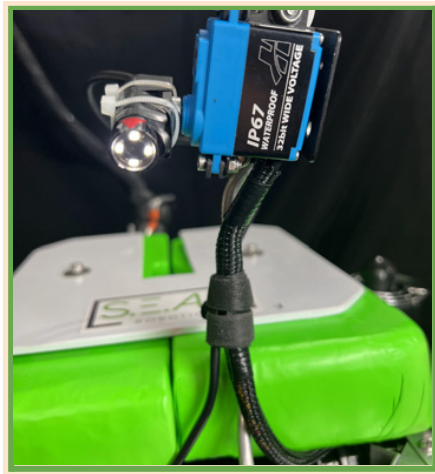
Figure 12: Camera mounted on flexible armature wire above the front gripper, which we refer to as a “birds eye” camera. The servo allows the camera to tilt or pan, greatly increasing the field of view.
