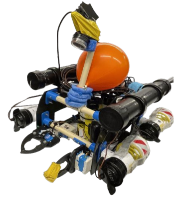
Figure 17: Variable Ballast System in Action Photo Credit: Ms. Barrett
