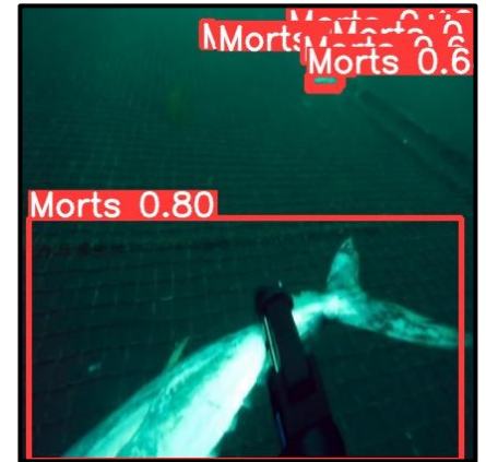
Figure 21: Test photo of AI Mort Detection Credit: Krithik
