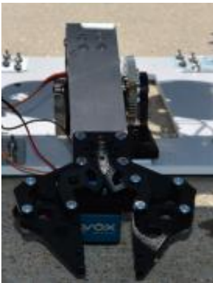
Figure 13: Assembled manipulator on base of frame.
