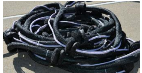
Figure 10: kraken's tether wrapped in black Tech and pool noodles added to make the tether neutrally buoyant.
