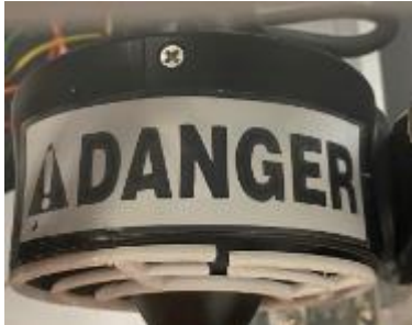
Figure 16: Danger labels on thrusters to warn operators of moving propeller parts.
