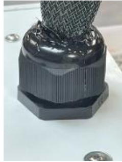
Figure 8: Tether restraint on the ROV side.
