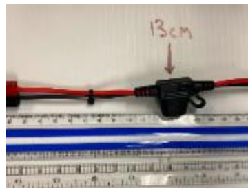
Figure 20: Safety fuse 13cm within main power line.
