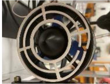
Figure 17: Guards on thrusters to prevent fingers from touching propellers.
