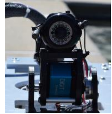
Figure 11: Main camera and tilt mechanism.
