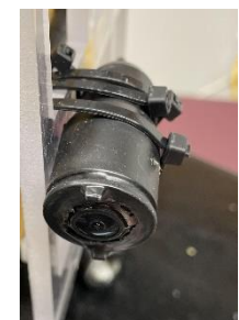
Figure 15: Waterproofed camera used on the ROV.
