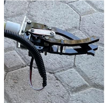
Figure 9: The 3-pronged claws utilized on the ROV.
