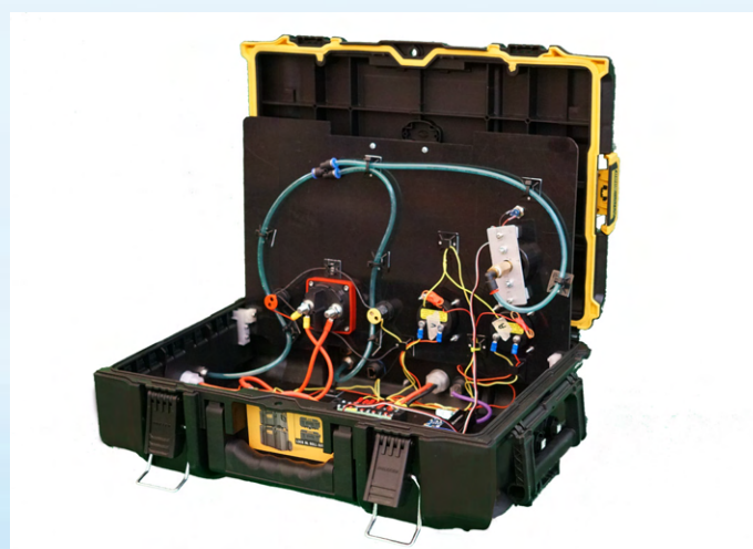
Figure 9. Beluga's Top-side Remote Piloting System (RPS) Photo by Lauren Jones
