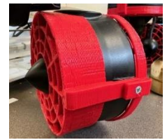
Photo 5: Thrusters with Shroud By: Allison Yu
