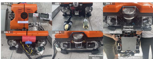
Figure 20. Six sides appearance of ROV for safety considerations.
