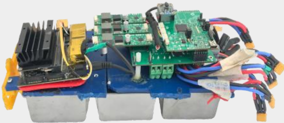
Fig 15 : 48-12V Converters and Electronics Housing
