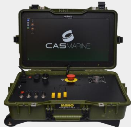
Fig 35: Surface Control Station
