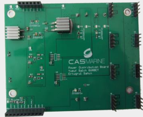
Fig 16 : CASMarine Power Distribution Board
