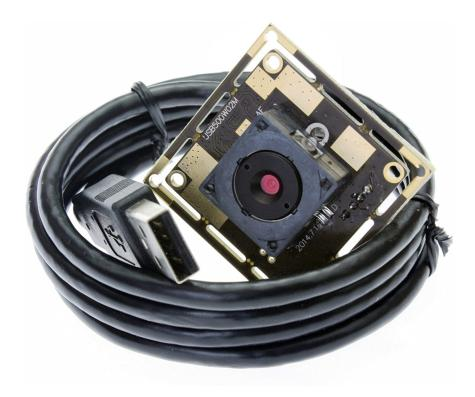
The ELP camera is a high resolution, auto-focusing camera with a max resolution of 2592x1944 at 15 frames per second.
