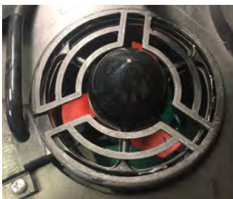
Picture 22 - Protective nets for propulsion
