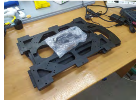
Picture 7 - Parts for frame assembly after CNC production
