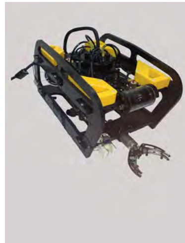
Picture 3 - Photo of the assembled ROV Tercel
