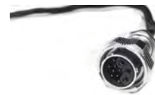
Picture 20 - Tether connector, control panel side.
