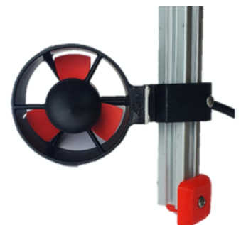
Figure 6: Thruster on the frame without shrouds
