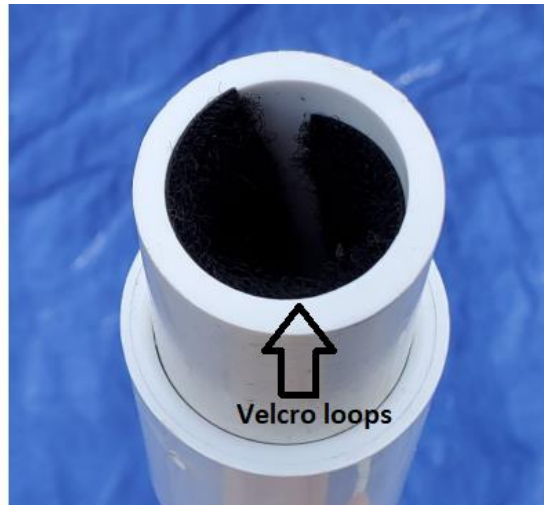
Left: 3" aluminum carabiner on the mooring connector. Three layers of tape on each side of the carabiner will prevent it from rolling against the ½-inch tee when secured with cable ties. Right: Velcro loops inside the 1-inch PVC coupling.
