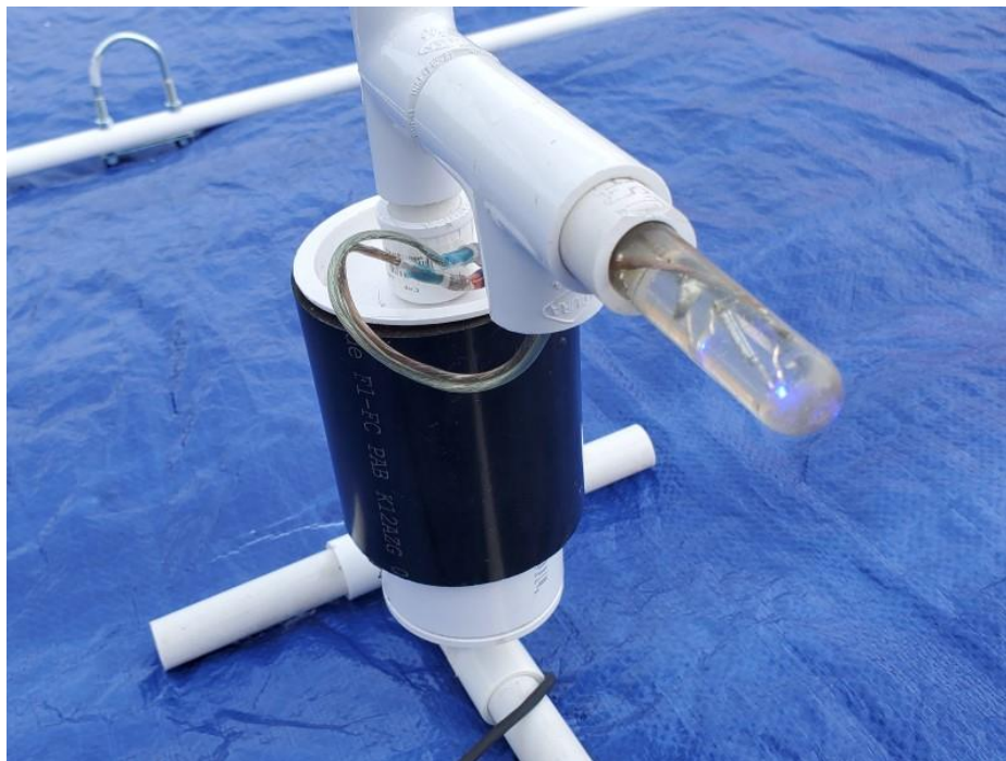
The power connector installed over the power port.
