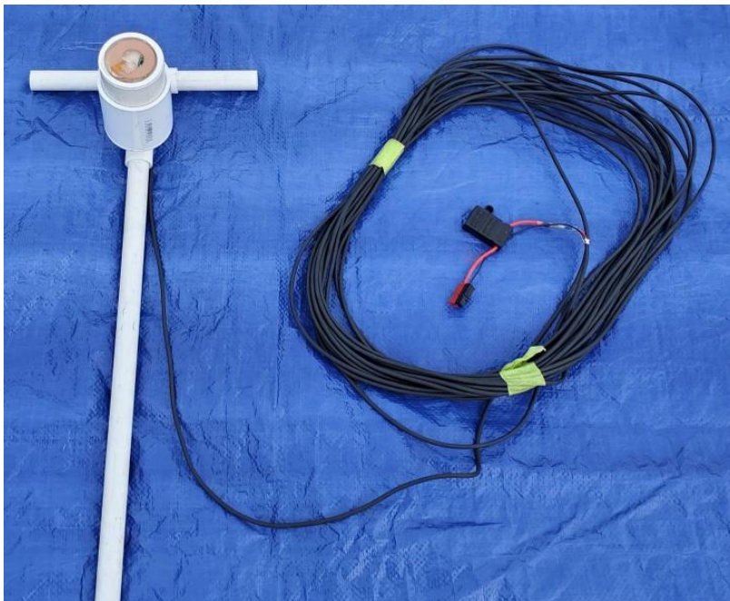
The MATE power port connects to a 12VDC power supply on the surface.
