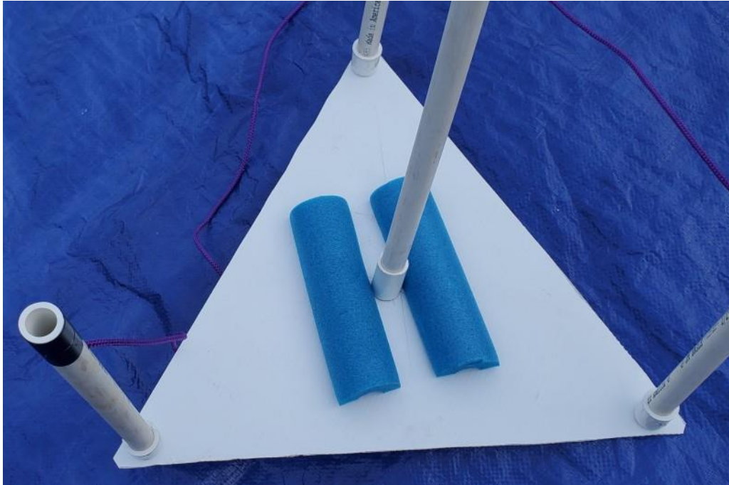
Flotation on the underside of the solar panel array.
