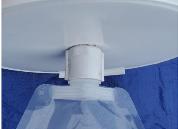
The 3/4-inch male adapter inserted through the hole in the 2-gallon bucket lid. Left: Top view. Right: Bottom view.
