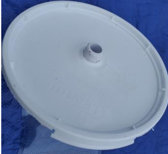
The 3/4-inch male adapter inserted through the hole in the 2-gallon bucket lid. Left: Top view. Right: Bottom view.
