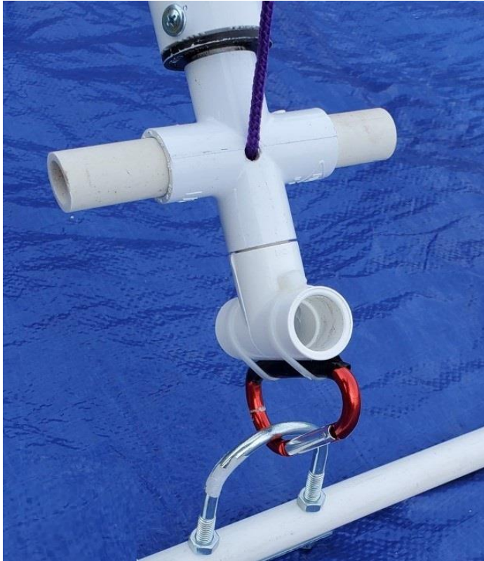
A mooring connector attached to an anchor point.
