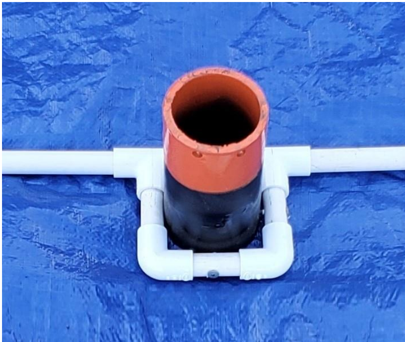
The power port is located in the center of the base framework and is constructed from 3-inch PVC pipe.
