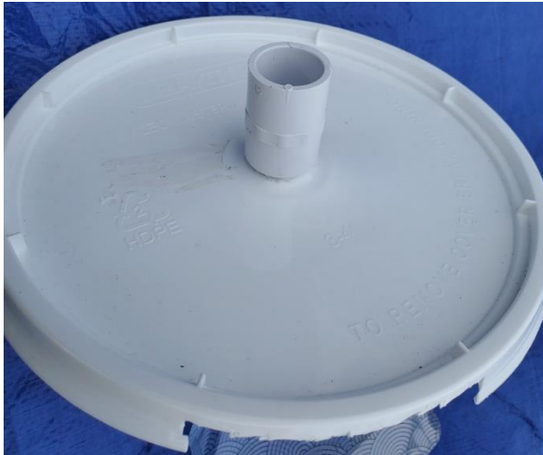
Left: The \frac{3}{4} -inch female adapter attached. Right: Plastic cling wrap secured over the top of the \frac{3}{4} -inch female adapter.
