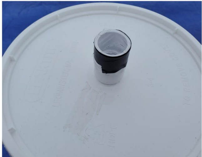
Left: The \frac{3}{4} -inch female adapter attached. Right: Plastic cling wrap secured over the top of the \frac{3}{4} -inch female adapter.
