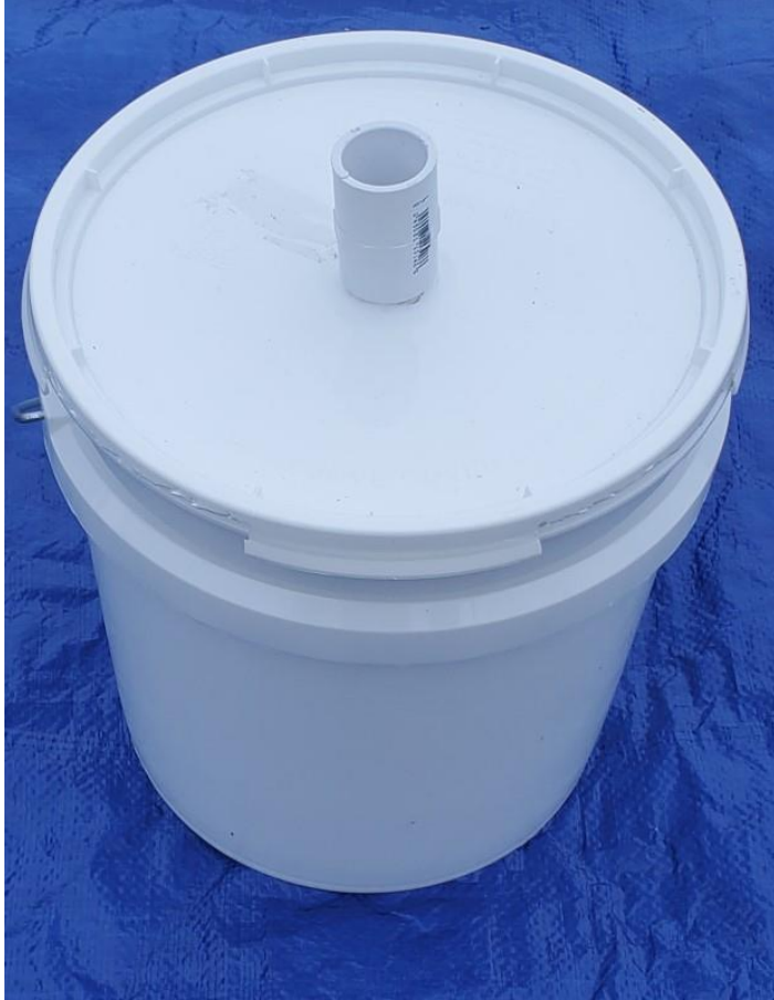
2-gallon bucket with lid attached. Weights are added inside the bucket.
