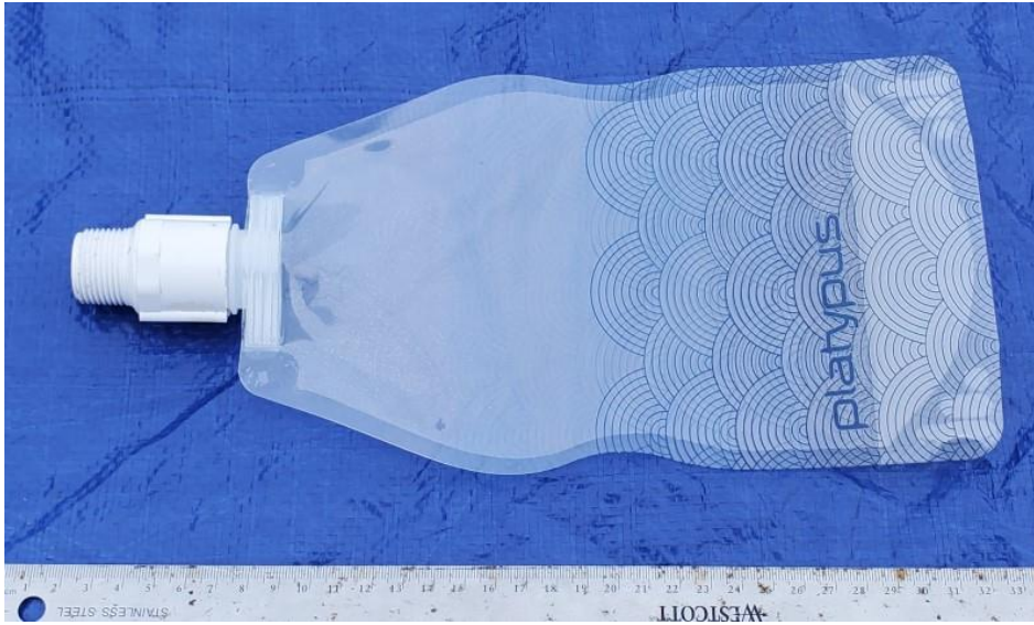
A 1 liter soft water bottle . Epoxy is used to secure a 3/4-inch male adapter to the mouth of the bottle.
