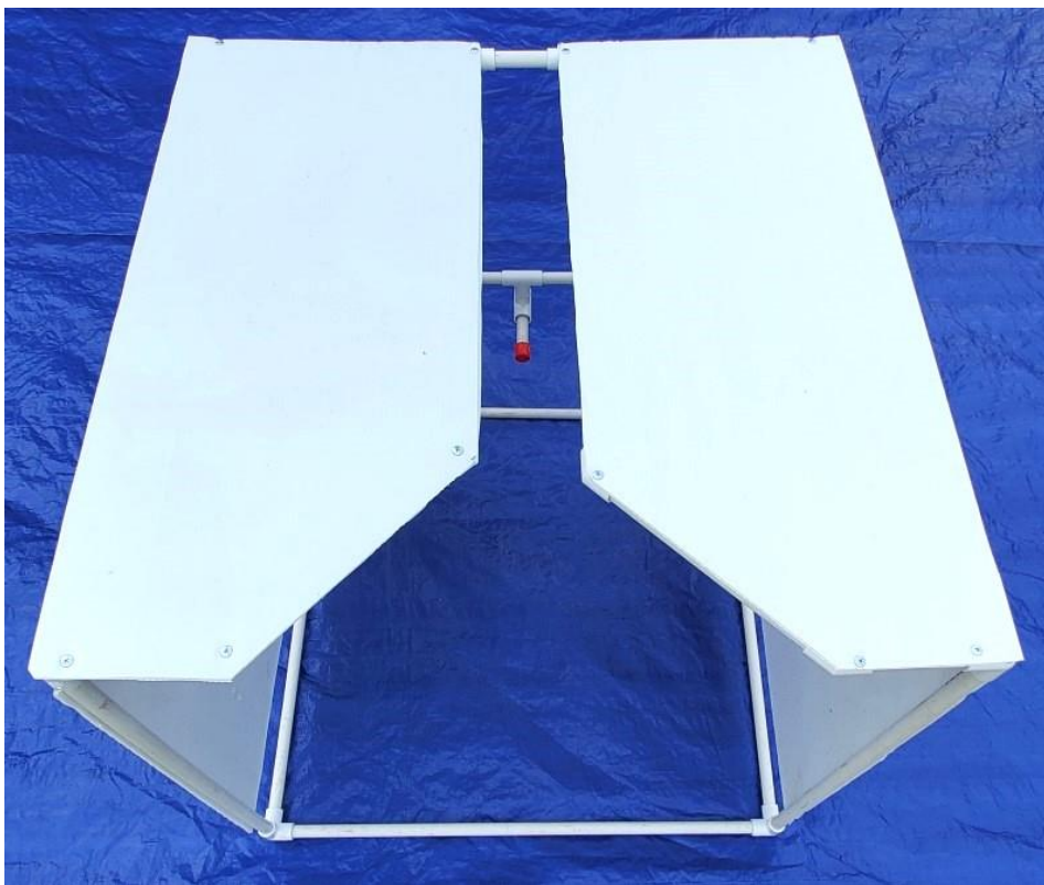
The docking bay with corrugated plastic sheeting attached.
