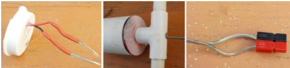
The transmitter side of the inductive coupling is attached to a wire that runs to the surface. Left: The solder connection is waterproof. Center: The wires pass through a hole in the ½-inch tee of the connector handle. Right: Anderson powerpole connectors are attached to the top end of the wire.
