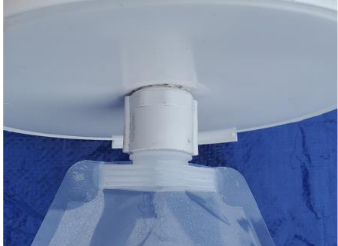
The \frac{3}{4} -inch male adapter inserted through the hole in the 2-gallon bucket lid. Left: Top view. Right: Bottom view.
