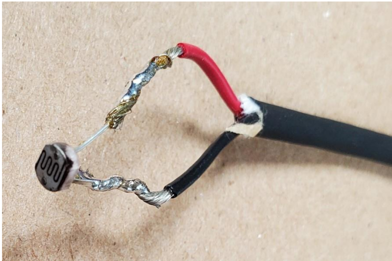
Left: The photoresistor soldered to wire. Right: The photoresistor wire through a hole in a 1-inch end cap.
