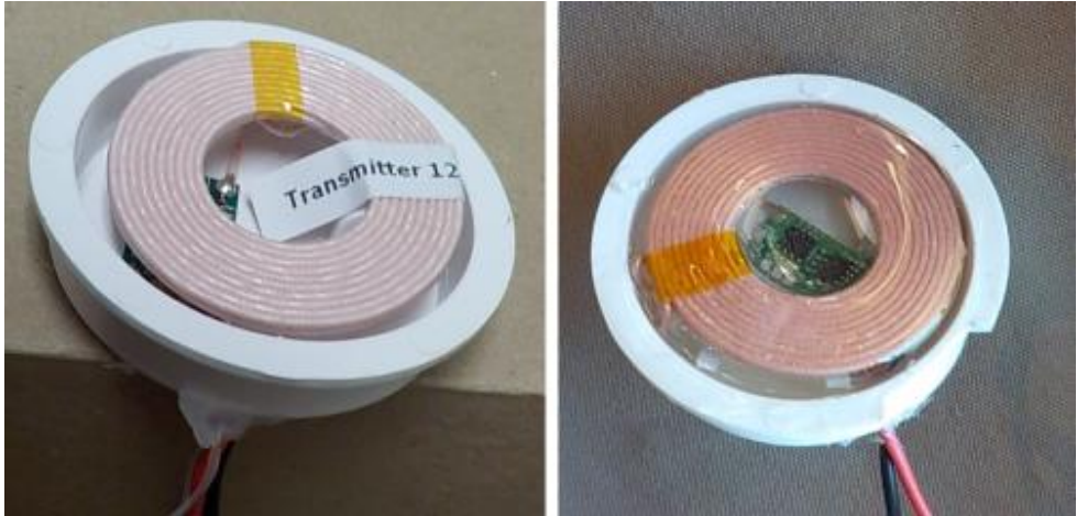
Left: The coil is raised above the electronics and flush with top of 2-inch knockout cap. Right: The coil is waterproofed with a slow curing epoxy ( Envirotext Lite ).
