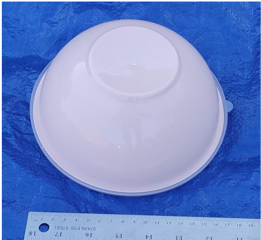
The coral head for probiotics is constructed from a plastic bowl. Weight inside the lid will make the coral head negatively buoyant. Design note: Open the lid when the bowl is underwater so that it fills with water.
