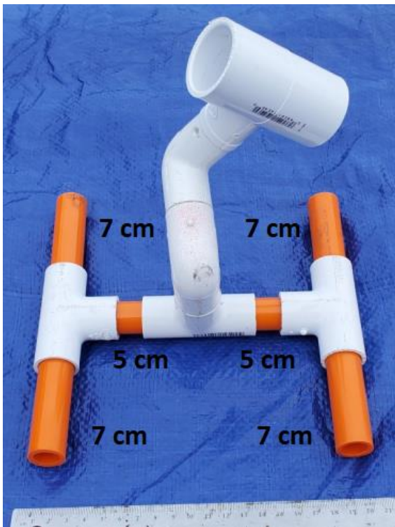
Left: Camera front view constructed from 1/2-inch PVC pipe. Right: Camera side view.
