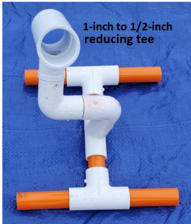
Left: Camera front view constructed from 1/2-inch PVC pipe. Right: Camera side view.
