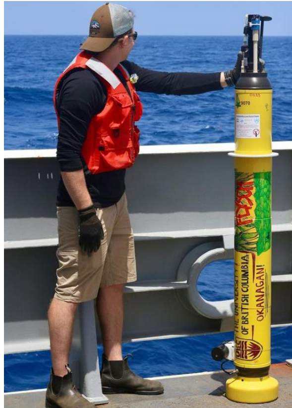
Readying a GO-BGC float for deployment ( GO-BGC | Global Ocean Biogeochemistry Array )
