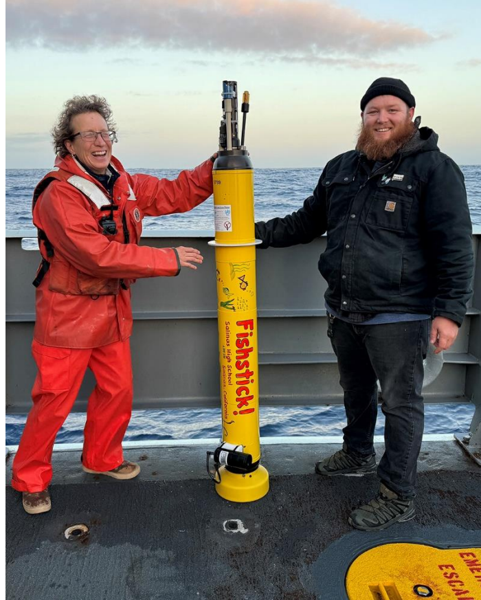
Readying a GO-BGC float for deployment ( GO-BGC | Global Ocean Biogeochemistry Array )
