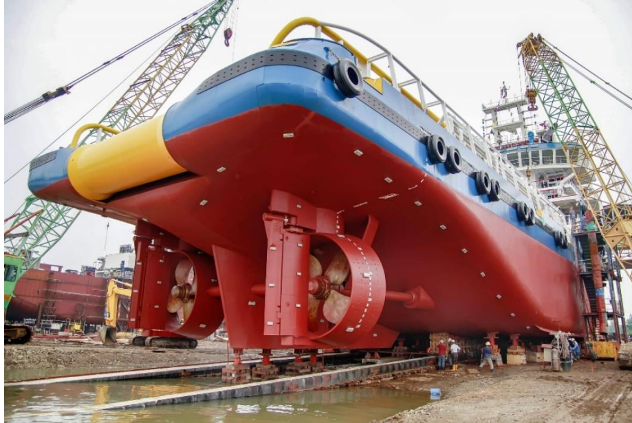
Sacrificial anodes attached to a ship's hull ( Sacrificial anodes - Cathwell )
