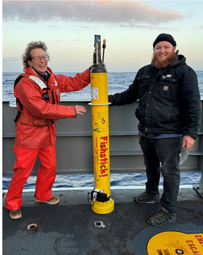
Readying a GO-BGC float for deployment ( GO-BGC | Global Ocean Biogeochemistry Array )
