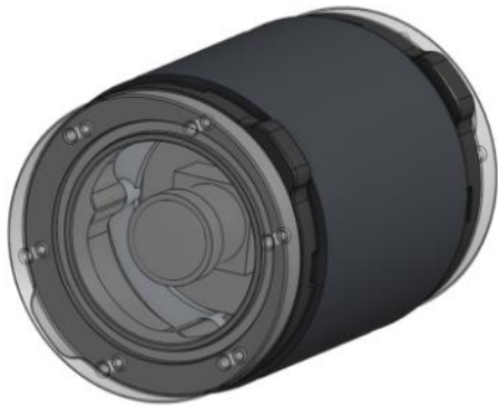
Figure 5.4 Camera housings. The main frame camera uses a serviceable O-ring enclosure, while the arm camera uses a compact potted housing for manipulator visibility.
